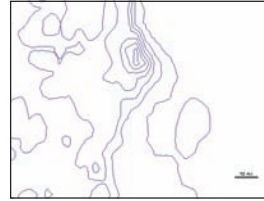
The contour interval is too large to show definition in the surface.
