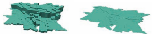
If the vertical exaggeration is too small (right), the view doesn't show enough variation.
